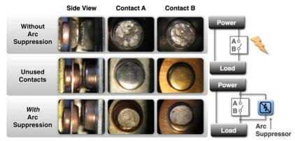
The pictures above show how use of a NOsparc<sup>®</sup> MHXAC contact arc suppressor can keep contact points in nearly new condition. In fact, arc suppression both improves relay operation and extends the inevitable end-of-life of a standard relay, contactor or snap action switch by a factor of 100 times or more under normal, specified relay operating conditions (please refer to the relay or contactor specifications).
