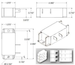
**NOTE:** Units may be stacked up to three (3) units high by threading a #6 screw through the mounting holes in the flanges..
