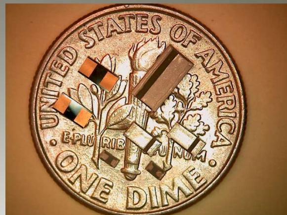
The Thermal Jumpers can be mounted between the chassis (or flange) of the heat source and an external heat sink providing a conduction path for the heat transfer creating a design alternative for systems where temperature cannot be controlled by forcing mechanisms like fans or water cooling systems.
